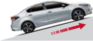
Hill-start Assist Control (HAC) (SX and Sports only) By maintaining brake grip until you step on the accelerator, HAC prevents the vehicle from dangerously rolling backwards when pulling away from a standstill on an incline.
