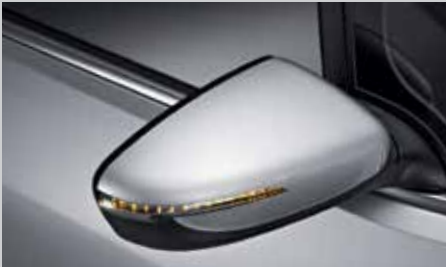
Wing mirrors with LED side repeaters The LED side repeaters in the aerodynamically-shaped wing mirrors let other drivers know your intentions clearly.
