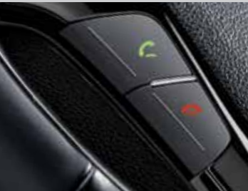
Steering wheel hands-free control (SX and Sports only) Conveniently located Bluetooth-hands free control switches allow you to make phone calls while remaining focused on the road.
