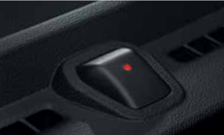
Security indicator A security indicator with blinking LED deters potential intruders with an automatic alarm system.
