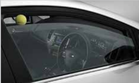
Safety power windows A safety mechanism built into the front windows prevent them from closing when an obstruction is detected.
