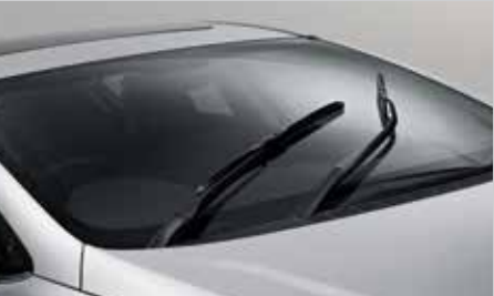
Aero blade wipers The wiper blades are aerodynamically designed to prevent them from lifting off the windscreen at high speeds.
