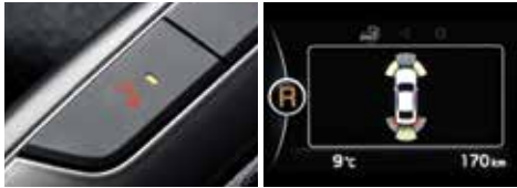
Front and rear parking assist system (SX and Sports only) Activated by a switch on the centre console, the front and rear parking assist system shows the distance between the car and any obstruction by means of a display on the supervision cluster.
