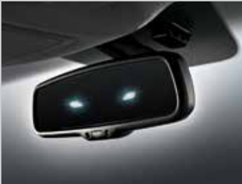
Electrochromic rear view mirror (Sports only) The mirror automatically dims to control the glare from the headlights of the vehicles behind during night time or low light driving conditions.
