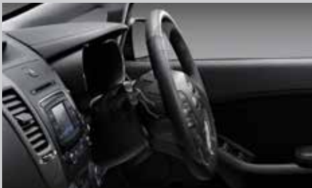
Manual tilt & telescopic steering column Adjust the position of the steering wheel vertically as well as backwards and forwards to suit your personal preference.
